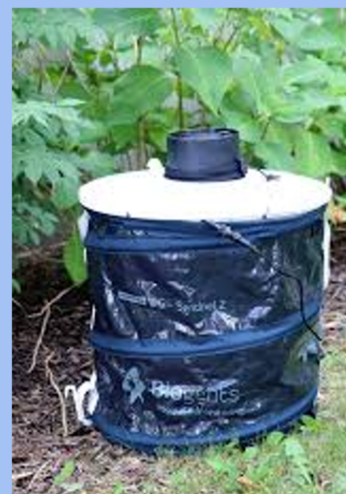
Figure 2: BG Sentinel 2 mosquito trap
