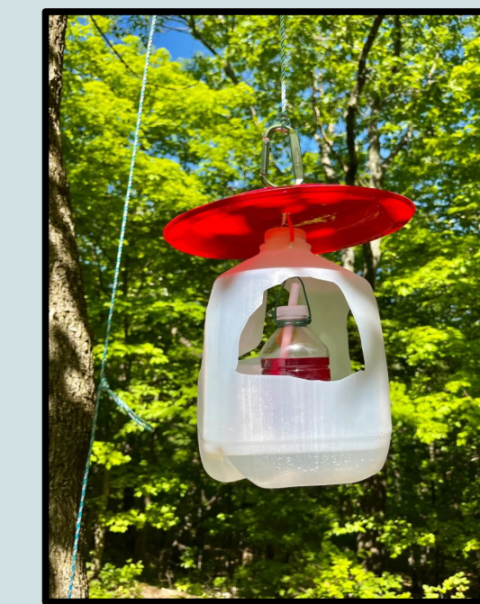
Figure 4: A common jug trap, note the openings on the sides.
