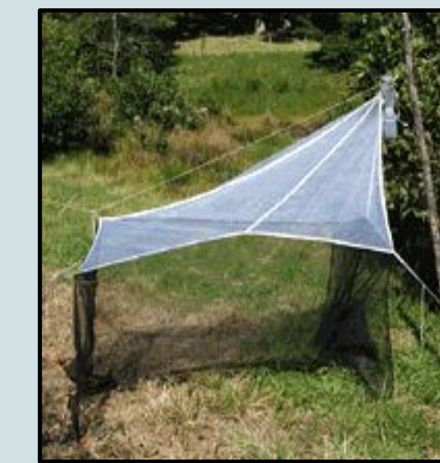
Figure 5: A common malaise trap, note the mesh walls.
