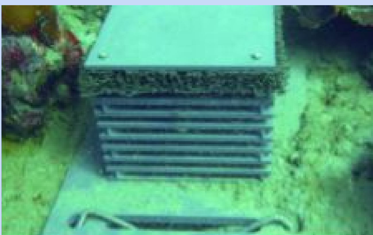
Figure 3. Autonomous Reef Monitoring Structure (ARMS) unit, composed of nine 23cm x 23cm PVC plates. Source: Smithsonian National Museum of Natural History
