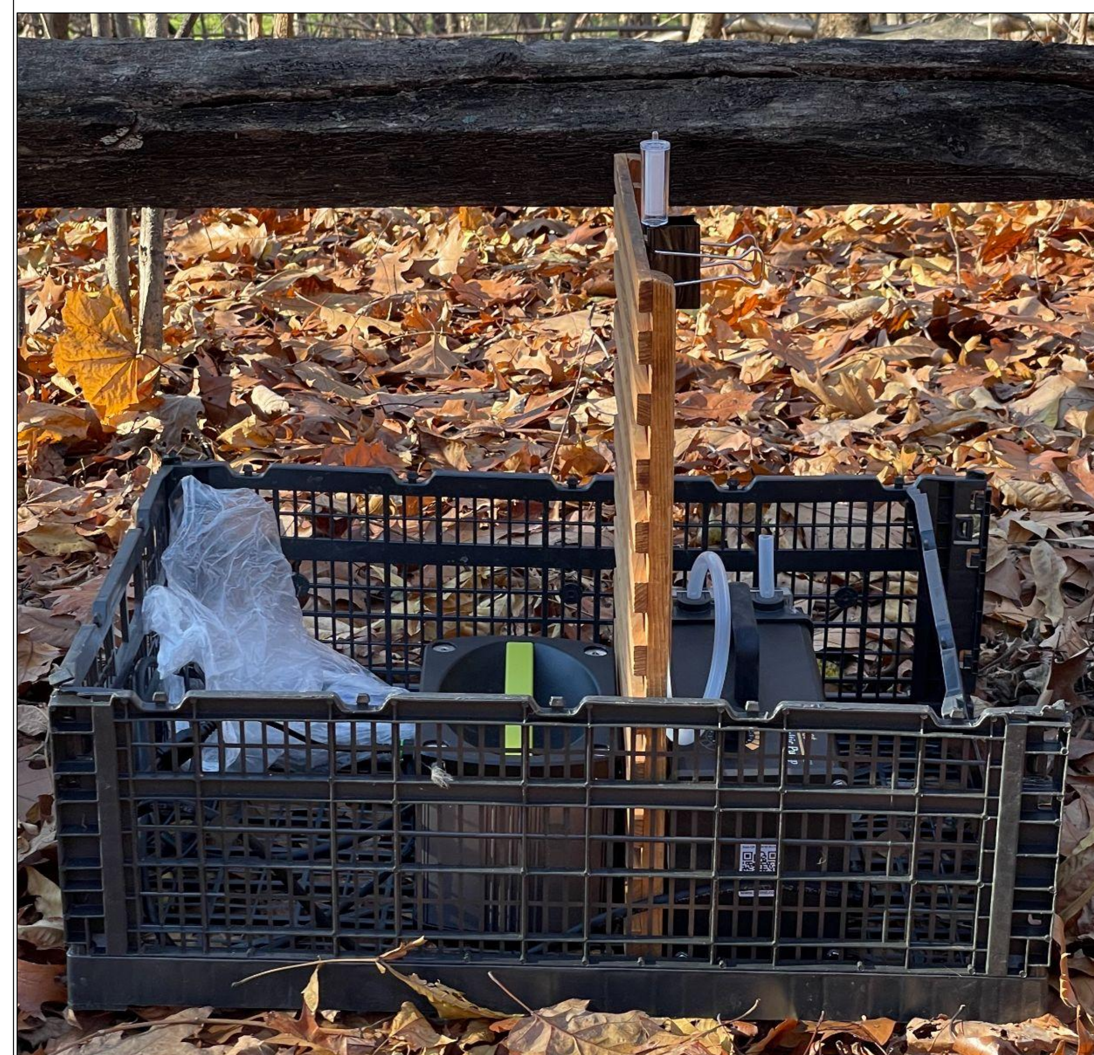
Fig. 2. Airborne eDNA collection Sterivex filter and pump.
