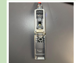
Figure 2: A MinION Mk1B or Mk1C device from Oxford Nanopore Technologies
